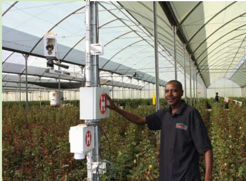
An optimum climate starts with measurements, so sensors are installed in the greenhouse.
