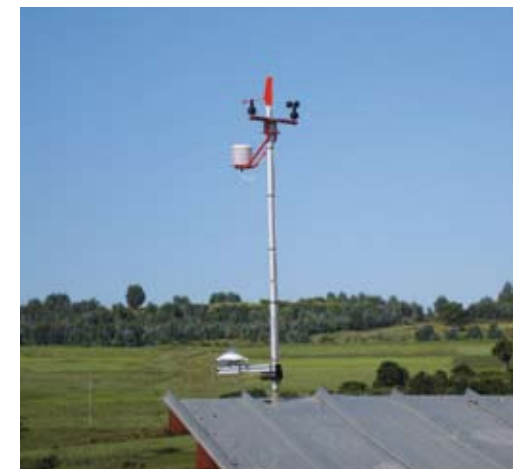
A weather station installed five meters above the greenhouse provides information on radiation, wind speed, outside temperature and humidity.
